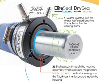
3) THE SEAL: Through the rotation of the shaft, injected water lifts the Lip Seal away from the shaft resulting in a thin layer of hydroplaning water between the fixed seal and rotating shaft. This hydroplaning prevents direct Nitrile Lip Seal contact while in motion (preventing dry rubbing and excessive friction wear). When shaft rotation slows, or stops, the hydroplaning action stops, and the seal returns to directly contact the shaft maintaining its dripless design.
